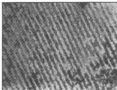
FIGURE 4 Permanent grating written with a single pump pulse observed under a polarised optical microscope. The grating period is \Lambda = 10 \mu\text{m} .
